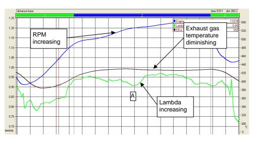
Figure 2. Plot of RPM, Lambda and EGT vs. distance
