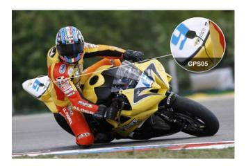
Install **GPS05 Module** near to the biker seat so that CAN cable (less sensitive to electromagnetic radiations) and not GPS antenna cable, passes near to the engine.
