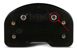
To connect **MXL Pro** connect **GPS05 Module** to the CAN cable labelled EXP (expansion) of the logger wiring.
