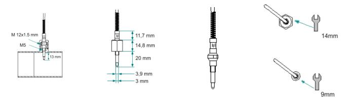
Below drawings show starting from the first on the left: EGT installation, its dimensions, a detail of the probe and the adjustable wrench to be used to tighten the EGT and the nut.
