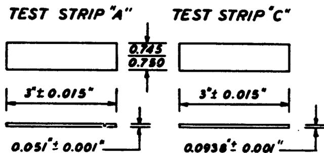
These strips of SAE1070 cold rolled spring steel are heat treated to 44-50  $R_c$  and must have a flatness of .0015 arc height as measured on the Almen Gage. It should be noted that practically all test strips purchasable today are about 46-48  $R_c$  and within 0.0005 arc height.
