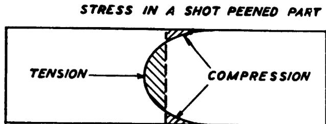
If the shot peened part is beam loaded, the stress which results is an additive combination of the stresses due to beam loading and the initial stresses due to shot peening as shown in following diagram.
