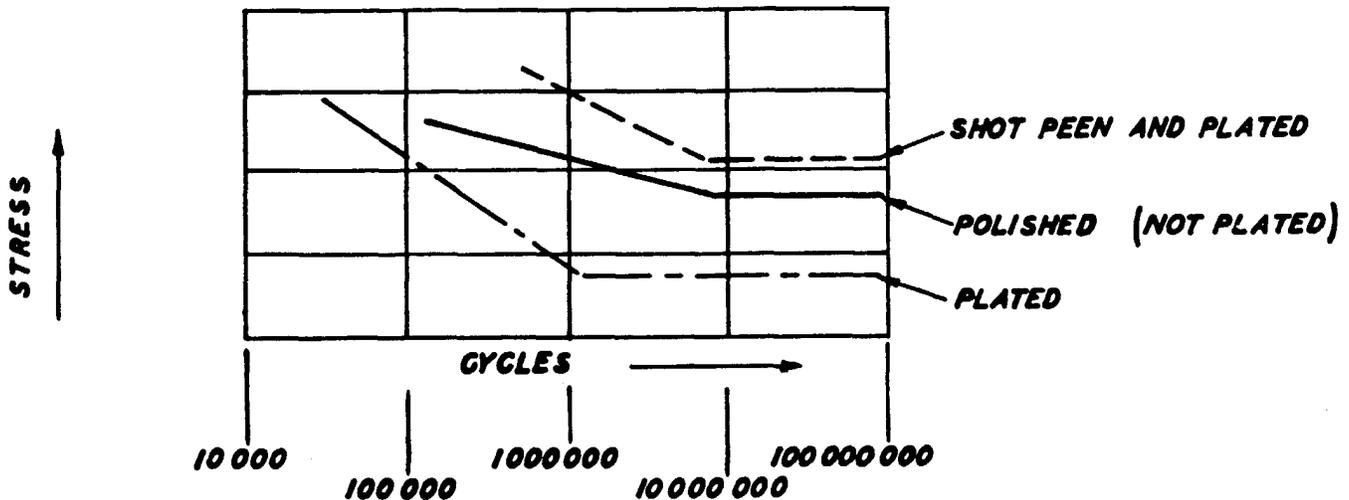
peening; however, shot peening will not improve a decarburized part to the point where it is as good as a properly heat treated part.
