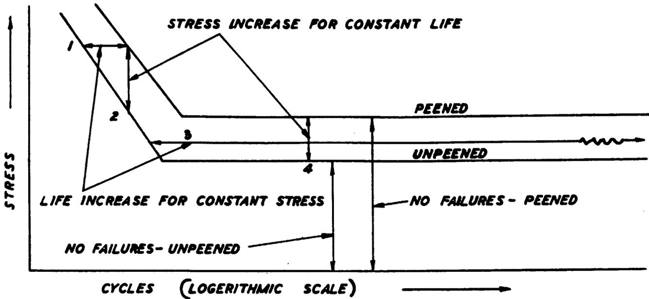
**HOW SHOT PEENING INCREASES FATIGUE STRENGTH AND LIFE**
