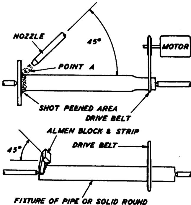
A dummy fixture (shown in lower part of drawing) would be made up which would rigidly hold an Almen block so that the distance from the center of rotation to the test strip would be the same as the distance from the axis of the shaft to point A which is halfway up the fillet. The block would be positioned so that its surface was at right angles to the blast stream when directly under it (45° angle to the axis of rotation). The fact that the ends of the Almen strip will come
