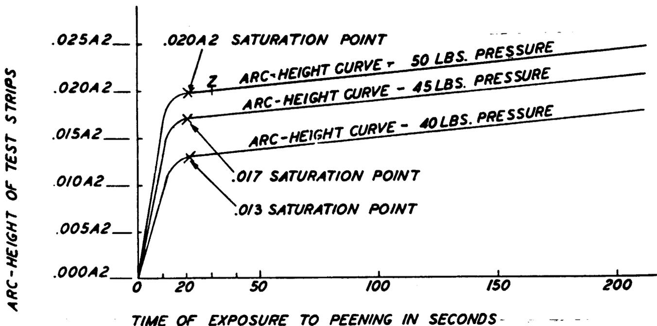
Almen strip and then shot peen it at this setting. The strip would be removed and examined under a magnifying glass and an estimate of the coverage (indented surface) made. In nearly all cases this will be above 90% at the saturation point. If it is not, we would repeat the foregoing tests using a smaller size shot and would find that we could get above 90% coverage by using say 40 pounds pressure and a peening time of 45 seconds to give us a saturation point arc height of .016A2.
