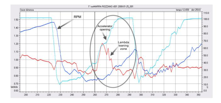
In red is shown Lambda course, in light blue TPS course and in dark blue RPM course. We would point out how, in the highlighted zone (throttle opening phase), Lambda course has some peaks upwards due to engine leaning.
