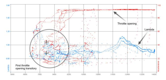
Accelerator value until a 100% value is red coloured while Lambda course on RPM value is blue coloured.
