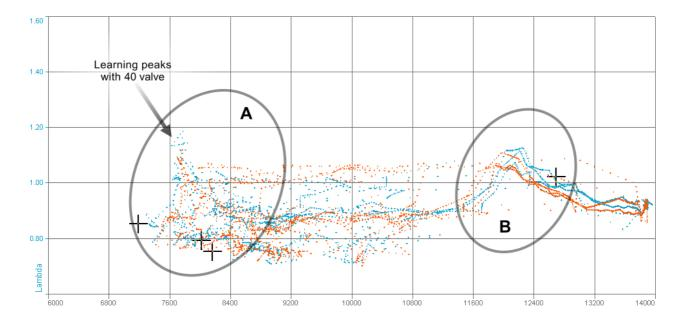
You can notice how in the highlighted zone there are no more engine leaning peaks. We still have to arrange the corner labelled as "B", around 12.000 RPM, that shows a peak in 100% throttle opening zone. To make this tuning we choose to mount a floating weighting 5,2, substituting that weighting 4 g.
