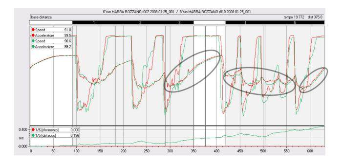
In red is shown speed and TPS course with the optimal carburetion, while in green are shown the same channels with standard carburetion.
