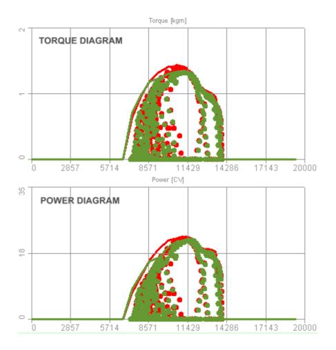
The red curve refers to the engine well carburetted while the green one refers to the engine with default carburetion supplied buy the manufacturer: please notice how a well done carburettor calibration leads to power gain.
