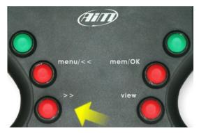
Using ">>" button, highlighted here above, it is possible to see on the right of the display fields 1 and 2 or 3 and 4 set in the software configuration.
