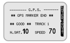
The message "GPS MARKER END" confirms that the procedure is ended successfully. "QUIT" ("VIEW" button) comes back to the main screen. In case during the setting there is a signal fall for any reason the display shows "GPS ERROR" and the procedure is to be repeated.
