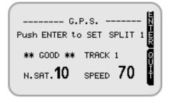
Use "ENTER" ("MEM/OK" button) to set splits. The display shows as many splits as have been set less one, to say if the dash is configured with 6 lap segments user is
